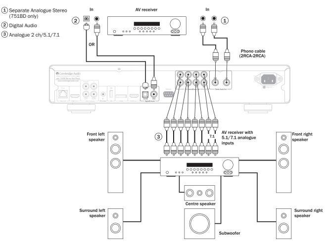
Speaker diagram shown for 5.1 channel setup. For 7.1 add two rear speakers.
